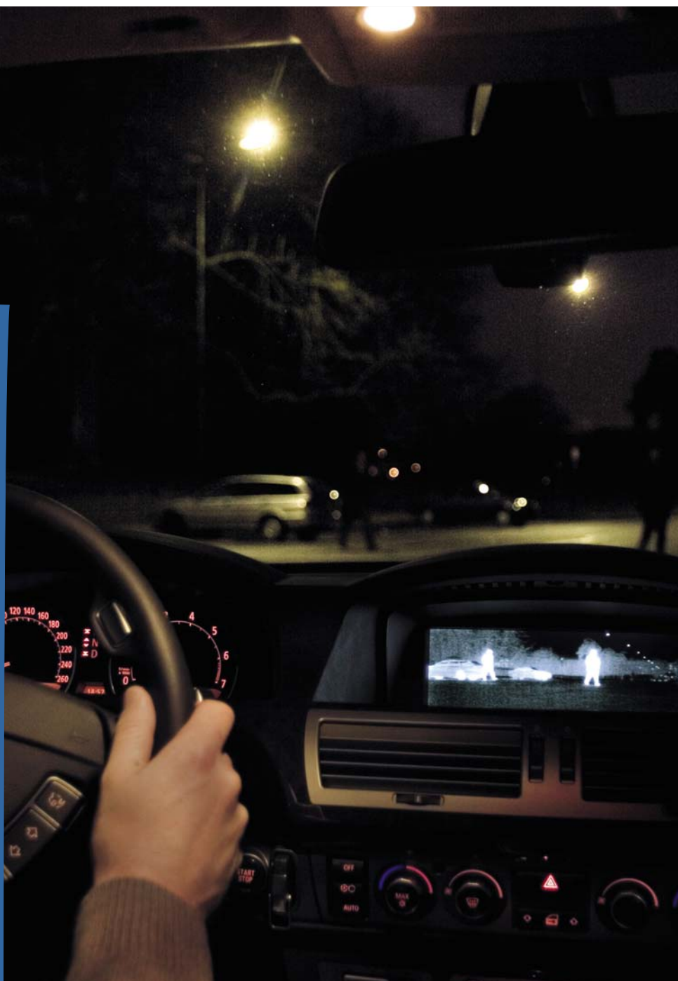
The night vision system which incorporates Umicore's GASIR lenses greatly enhances visibility at night
