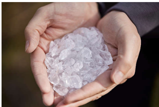
Production scraps from fiberoptic cables containing germanium
